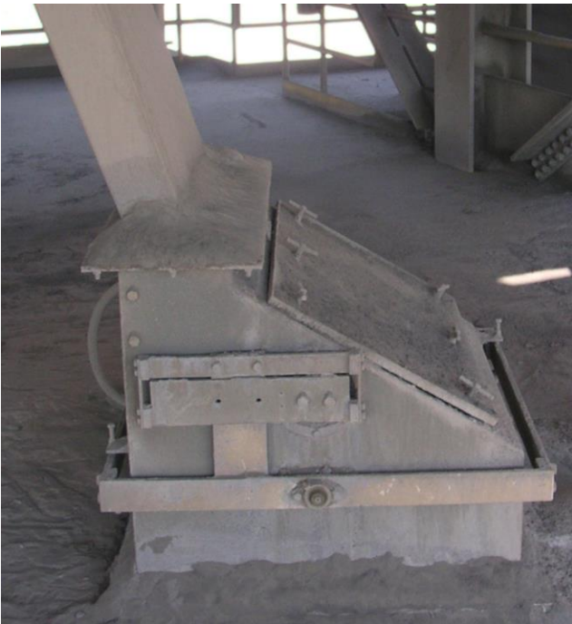
DLM Solids Flow Meter with a curved measuring chute receives material free of impact
