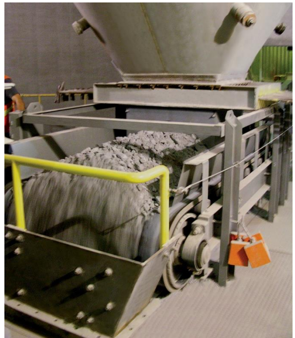
The DMO Weighfeeder is designed to feed silica, limestone, iron, fluff, TDF and numerous others
