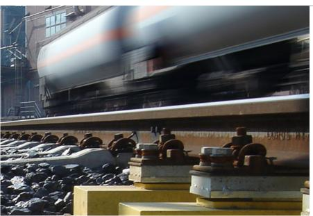
The new MULTIRAIL® LiquidWeight has been specially optimised for weighing liquids. The tested and certified system can weigh with precision almost any wagon type or complete block trains.
