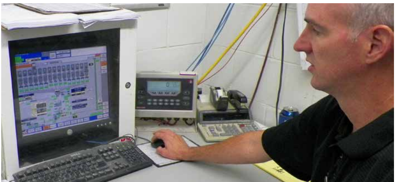
Brent Lortscher, president and project engineer at LASI, demonstrates how he can compare different material characteristics by displaying the hammermill power usage graphs for production runs manufactured weeks or months apart in the comfort of his own office.
