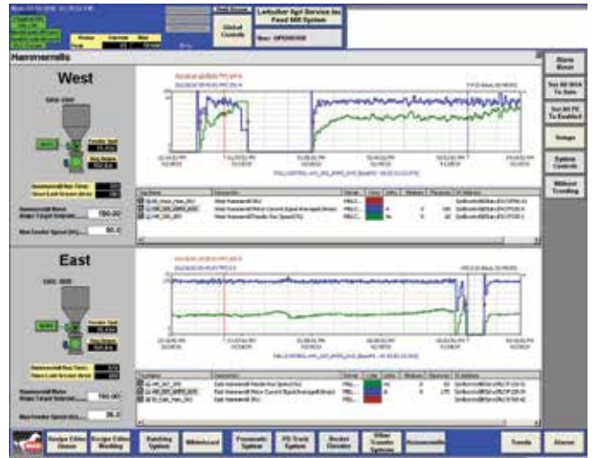
Mac Process ActiveFactory software provides a flexible front-end to the Historian database that allows users to view data in various formats, such as graphs and varying time spans.
