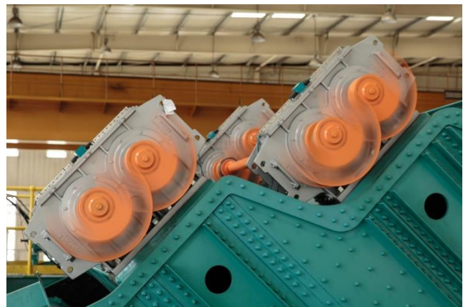
Picture: DF704 Exciters mounted in pairs on two exciter Beams.
