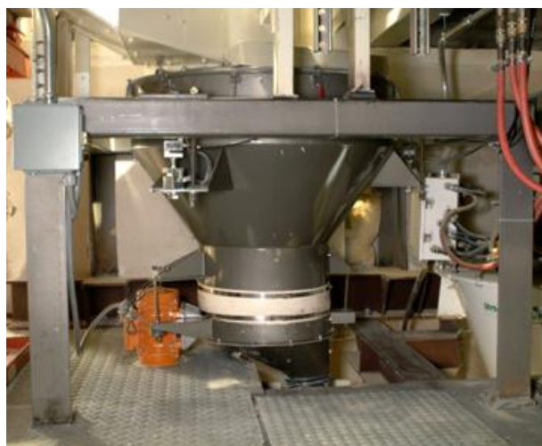
A vibratory feeder attached to the hopper's bottom induces material discharge.
