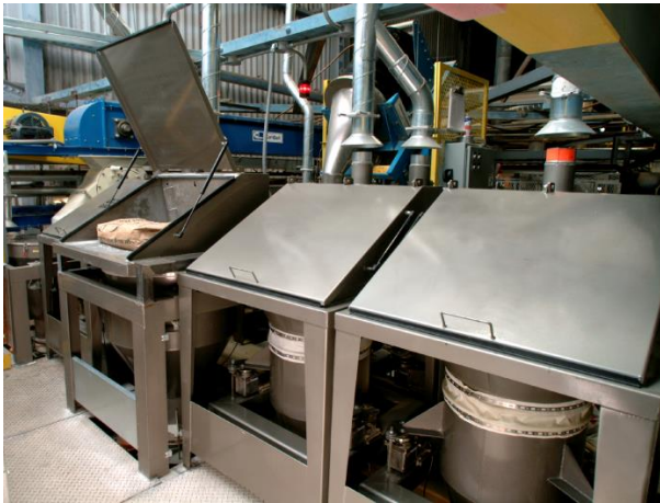
The bag dump stations are connected to the hopper's tops, allowing installation in areas with limited space
